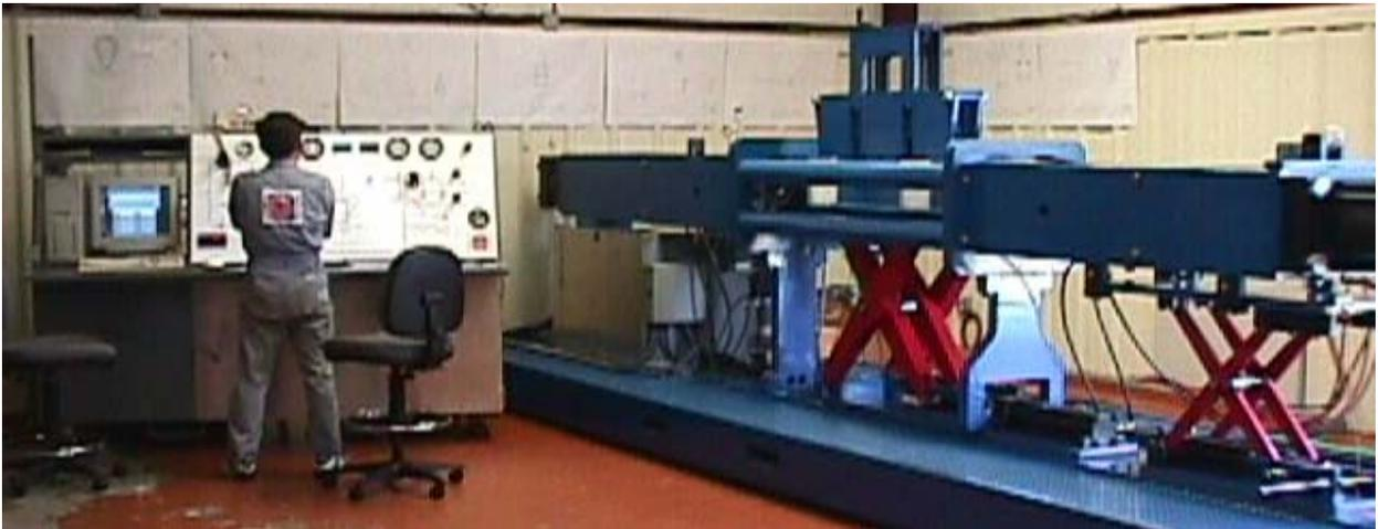
***Figure 30 – Coiled Tubing Test Machine***
