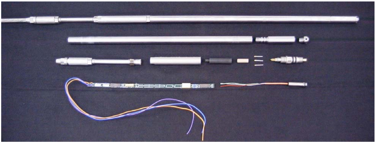
Figure 5.1 – 3/4" OD Downhole Pressure and Temperature Tool
