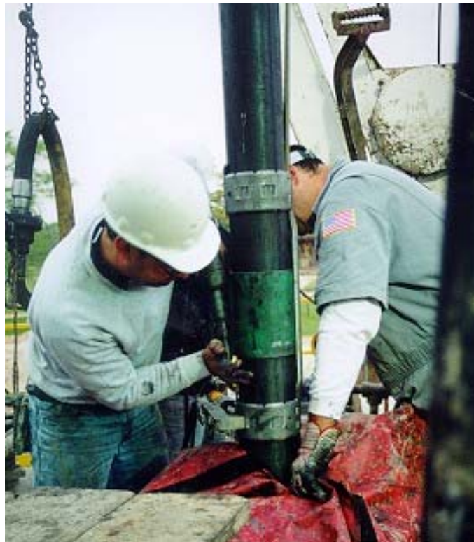
Figure 5.3 – Successful Strapping Method
