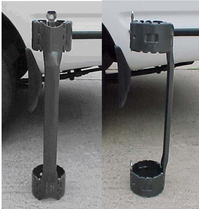
Figure 7.5 – Clamps used to attach cable and tools to casing
