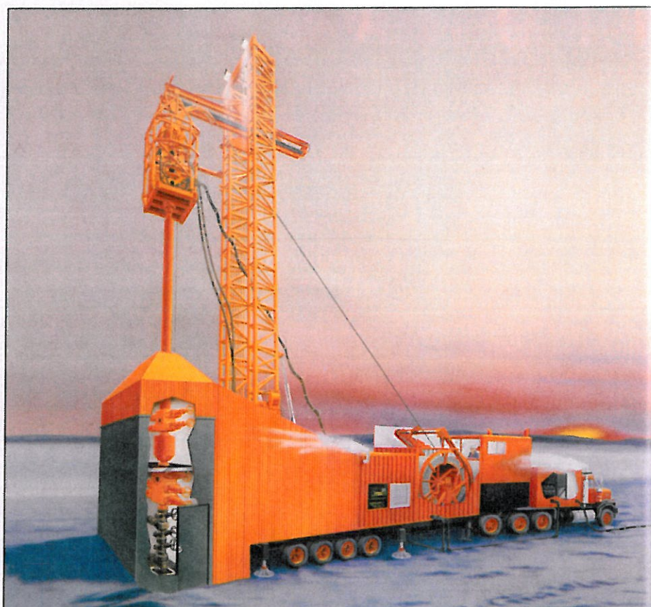
Fig. 1. A dedicated coiled tubing drilling unit, such as that depicted by this artist's rendering, is now being jointly designed by Arco and Dowell for Alaska's Prudhoe Bay.
