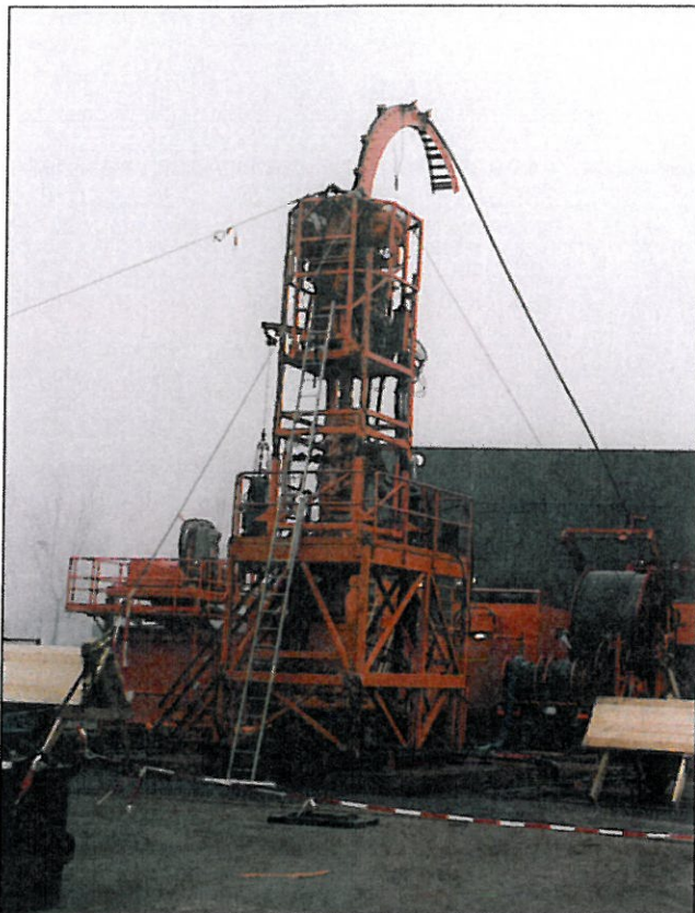
Fig. 2. Upon recompletion, NAM's Berkel No. 5 well produced eight times more oil on natural flow than it produced previously with the assistance of a beam pump.
