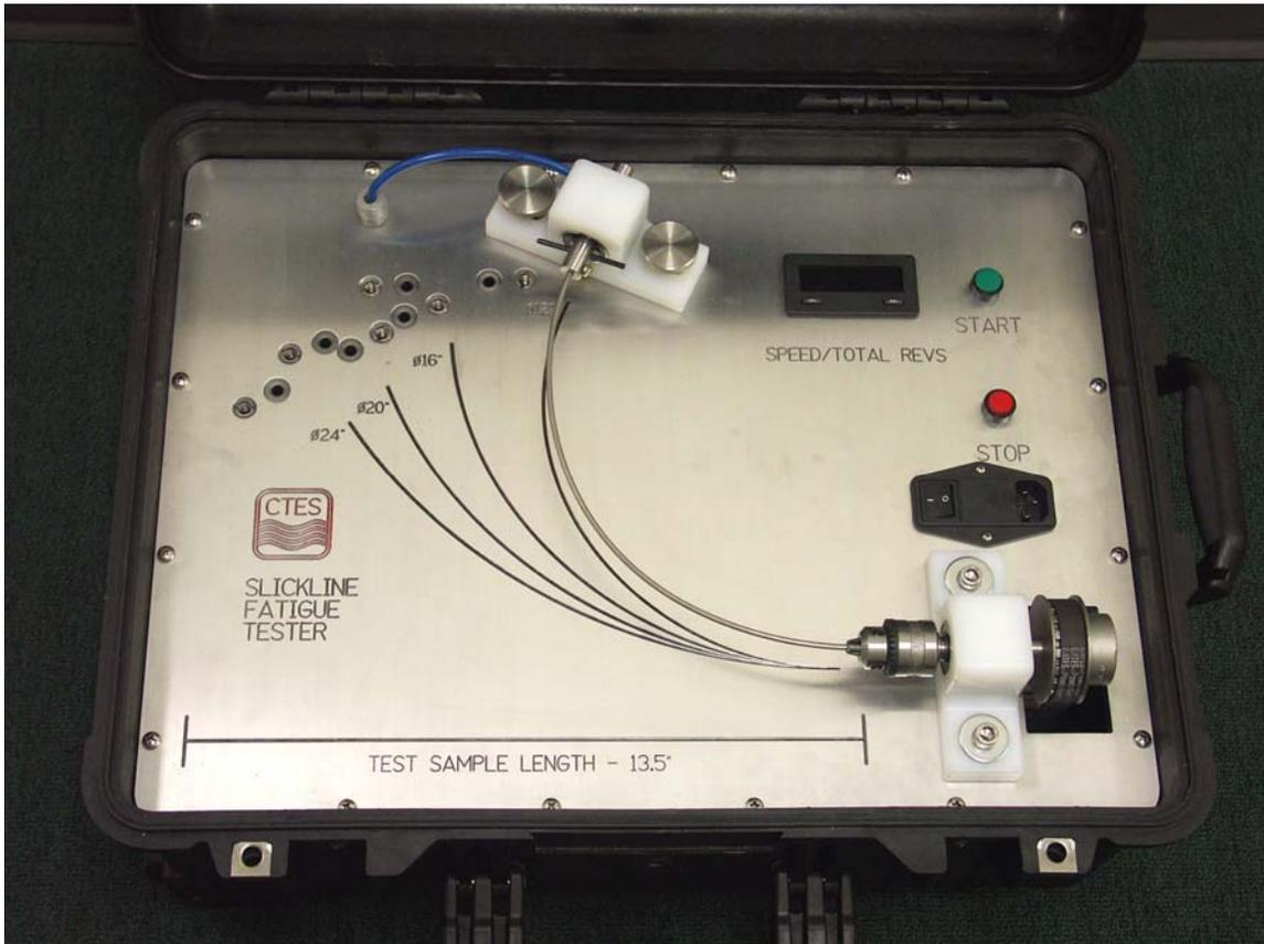
**Figure 8- Commercial Portable SL Fatigue Tester**
