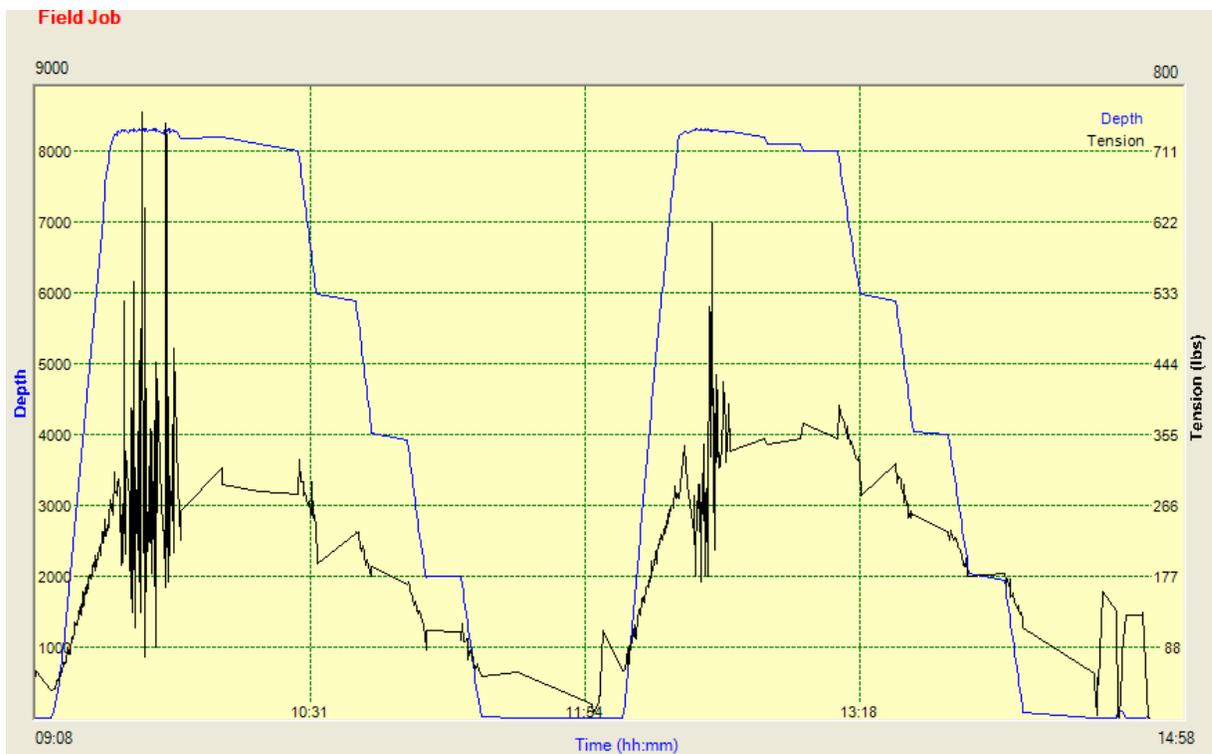
Figure 10- Typical Job Data from Data Acquisition System
