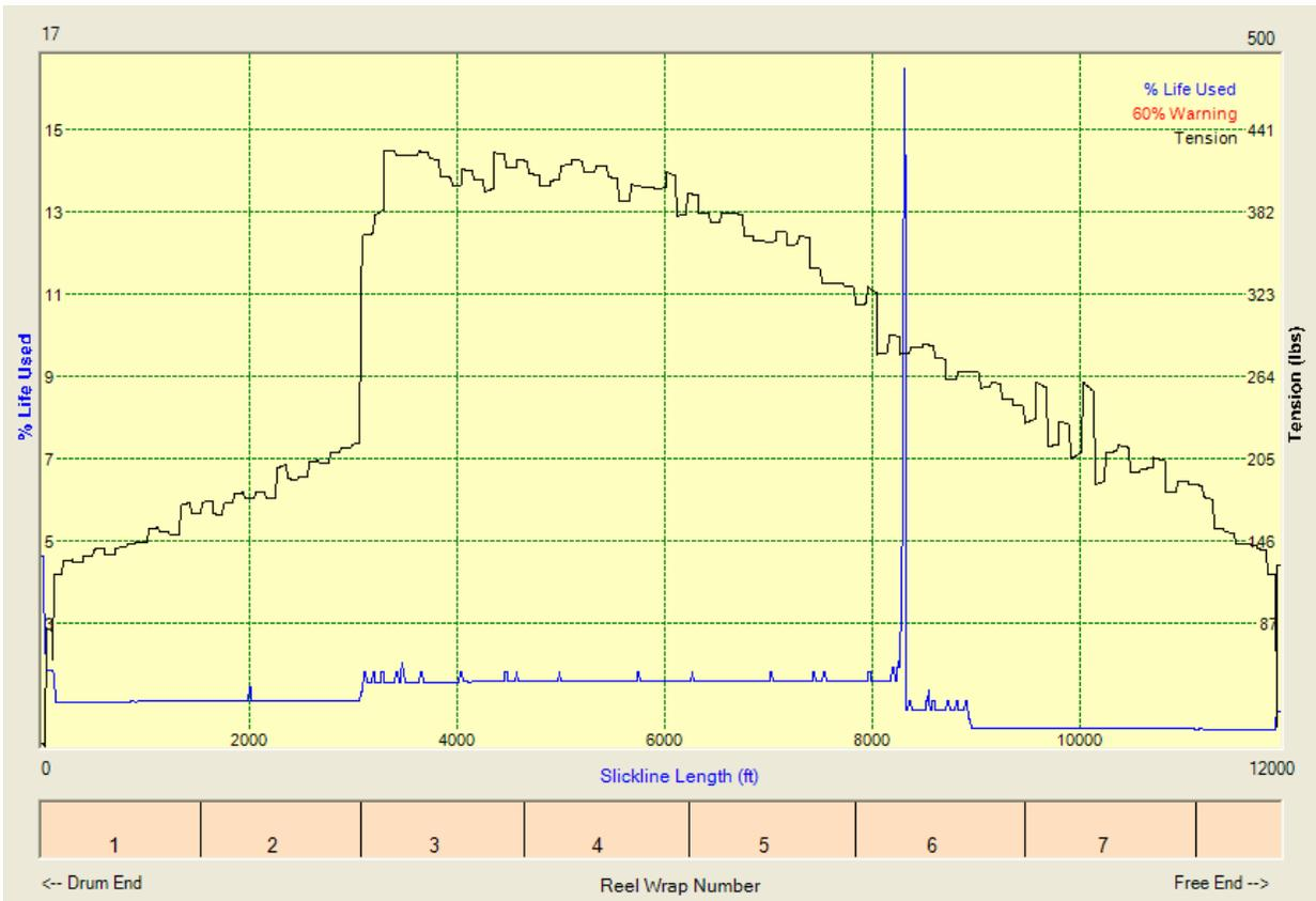
Figure 11 - %Fatigue Life Used and Tension vs Slickline Length
