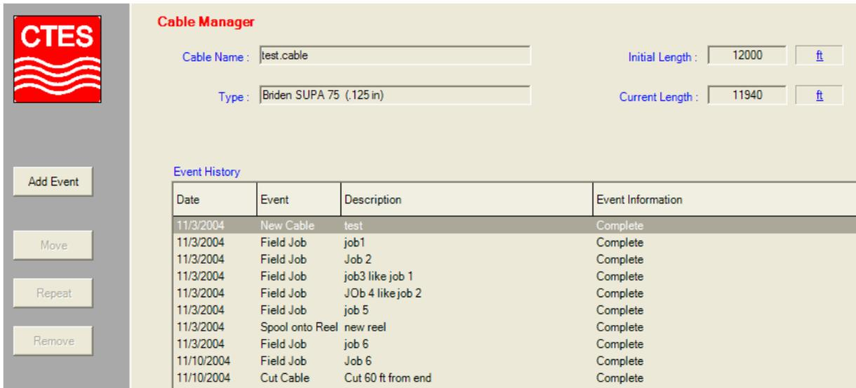
Figure 9 – Main Screen of Slickline Fatigue Tracking System
