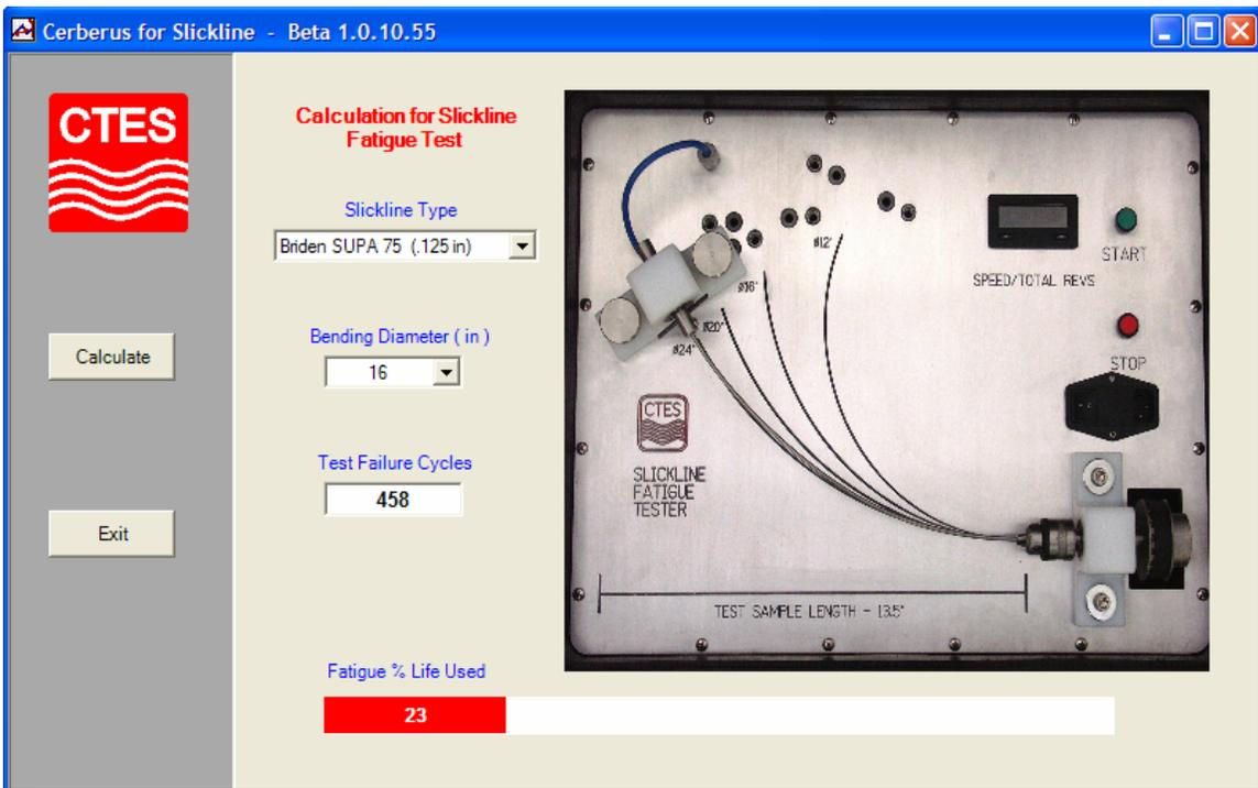
Figure 12 - %Fatigue Life Used for Field Test Sample
