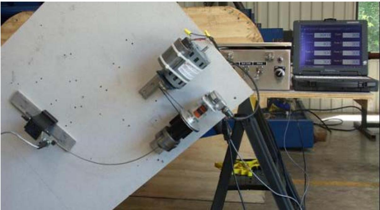
**Figure 4 - SL Fatigue Test Machine without Tension**
