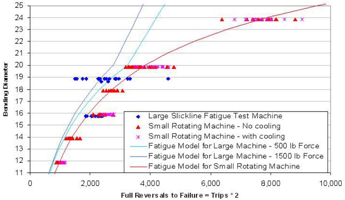
**Figure 7 - Fatigue Test Data and Model Results for Bridon SUPA75 0.125"**
