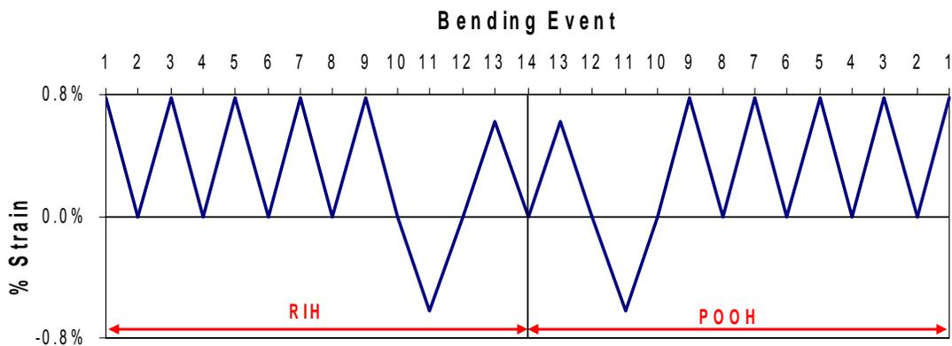
**Figure 2 – Strain for each Bending Event in a Typical Well-Site SL System**
