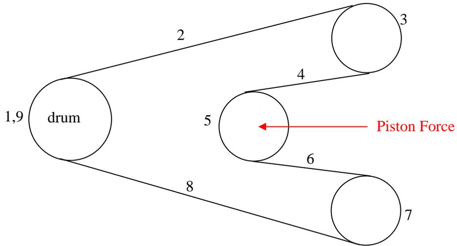
**Figure 5 – Schematic of Large SL Fatigue Test Machine**
