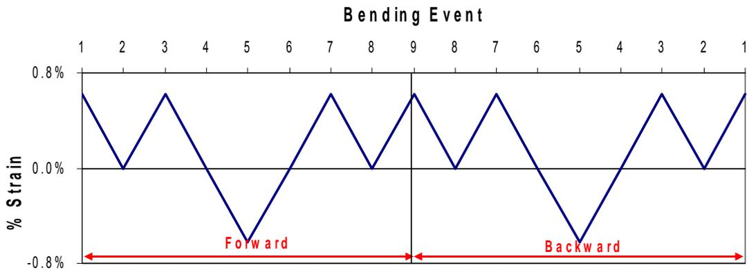
**Figure 6 - Strain for each Bending Event for the Large SL Fatigue Test Machine**
