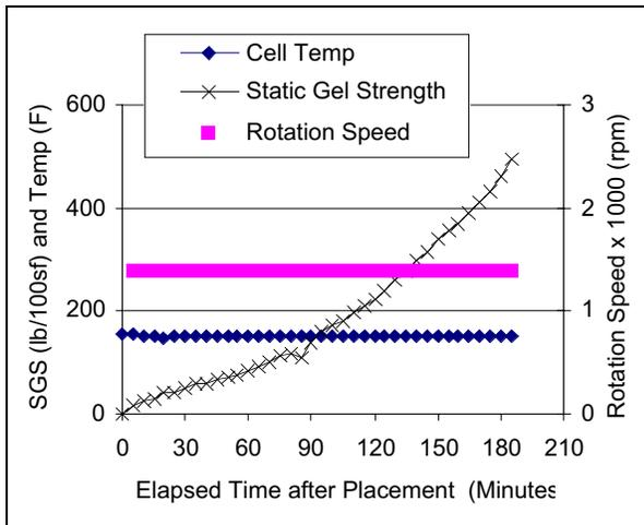
**Figure 2 - Static Gel Strength Test on Lead Slurry for Field Example**
