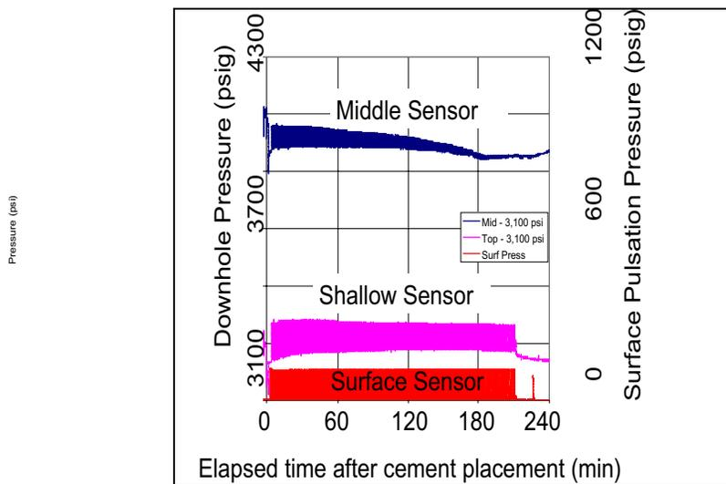
**Figure 1 - Pressure Pulsation Record for Field Example**
